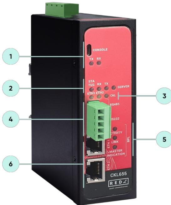
1. Micro USB or USB Type-C Console port for LOG in 115200 baud
