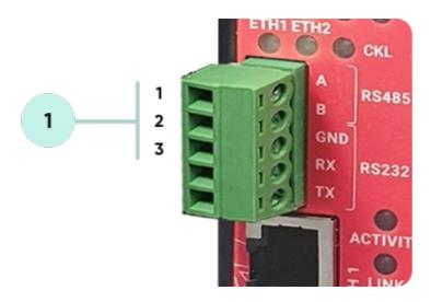
Terminal Connector for 2 wire RS485 connection and GND (if needed)
