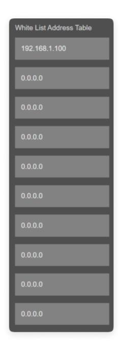
In this page user can enter 0.0.0.0 or the exact IP value of the device. The options with 0.0.0.0 will be disgarded ( not filtered).
