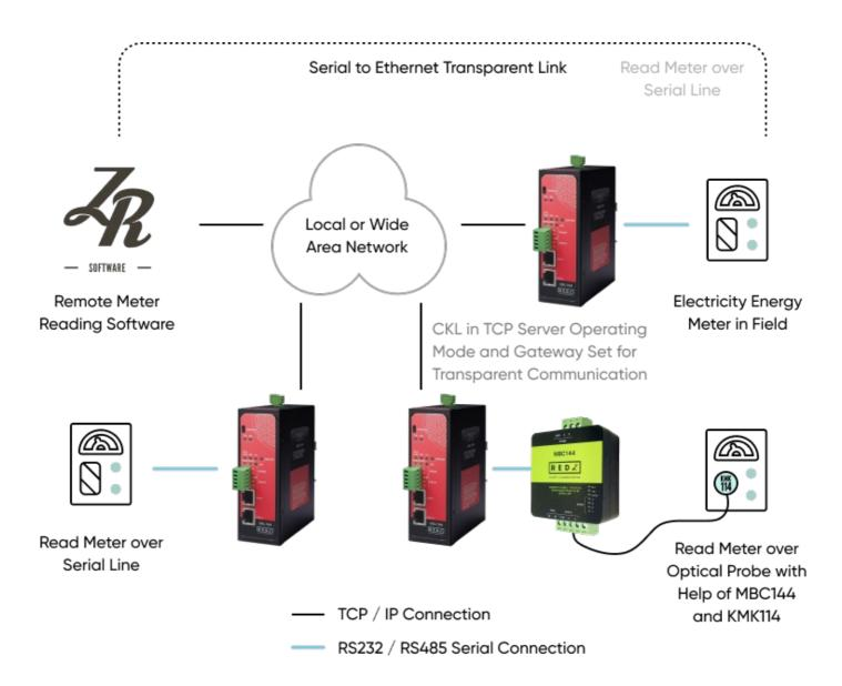
CKL Gateway devices in field configured for Transparent Communication and act as TCP Server to Serial Device Gateway. Field devices are connected over serial line either over RS232 or RS485 and communication data type and baud rate fixed.
