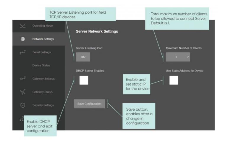
Following parameters and static IP settings available for "DHCP Server" setting.
