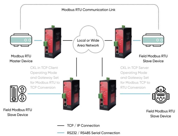
CKL Gateway device on Modbus RTU Master side configured for Modbus RTU to TCP Conversion and act as TCP Client to Serial Device Gateway. Field devices are defined as a list in configuration to enable mapping with field devices Modbus Addresses and related CKL remote fixed TCP IPs and ports.
