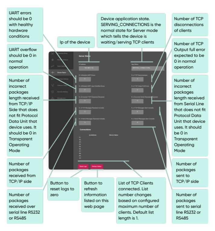
After clicking "Refresh Status" button, system will reload data only and will not reload page. Button will be disabled during reload for an instance. If timeout occurs during the reload, the button will be enabled again with warning of timeout. In normal operation reload of status data will be
