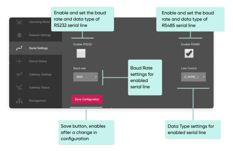
Once the setting has been changed, "Save Configuration" button will be enabled.
