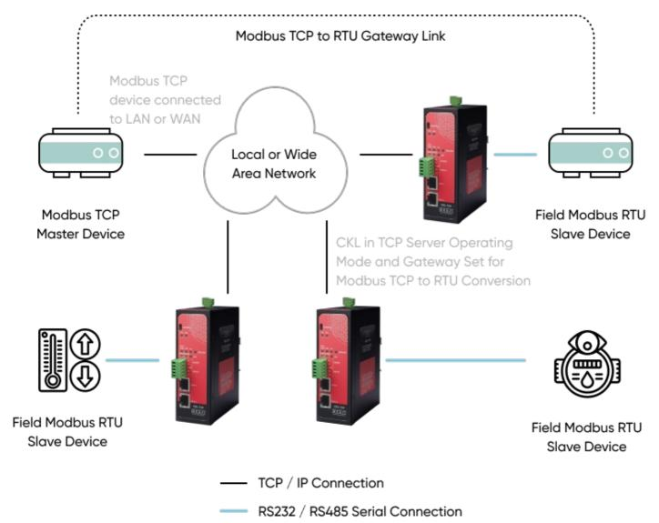
CKL Gateway devices in field configured for Modbus TCP to RTU Conversion and act as TCP Server to Serial Device Gateway. Field devices are connected over serial line either over RS232 or RS485 and communication data type and baud rate fixed.
