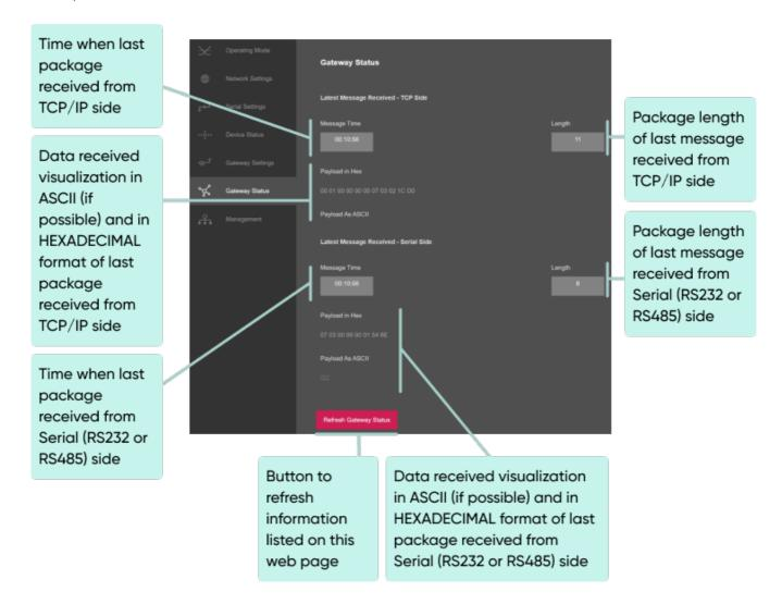
After clicking "Refresh Gateway Status" button, system will reload data only and will not reload page. Button will be disabled during reload for an instance. If timeout occurs during the reload, the button will be enabled again with warning of timeout. In normal operation reload of status data will be done immediately.
