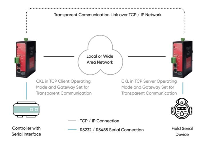
CKL Gateway device in Controller side configured for Transparent Communication and act as TCP Client to Serial Device Gateway. Field device is connected over serial line either over RS232 or RS485 and communication data type and baud rate fixed. CKL can connect to Other CKL device on sensor side by manual entering the IP of TCP Server or simply using REDZ special design, plug and play Server-Client Operating Modes.
