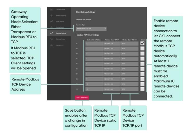
Once the setting has been changed, "Save Configuration" button will be enabled.
