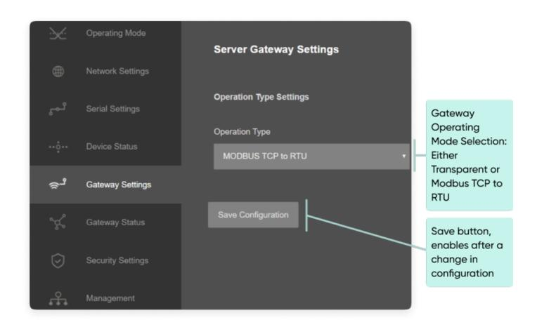
Once the setting has been changed, "Save Configuration" button will be enabled.
