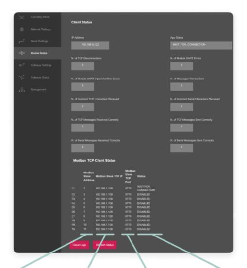
Column shows the configured Modbus Address for the remote Modbus device Column shows the configured static TCP IP for the remote Modbus device
