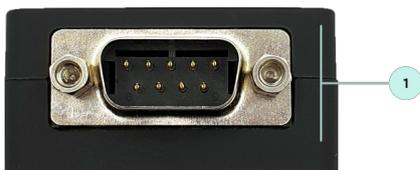
1. DB9 Male connector for RS232: Only Tx-Rx-GND for data transmission.
