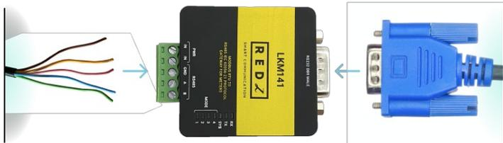
Modbus RTU Plug and Play version can directly fit into EMH LZQJ-XC meter. It is direct replacement for Variomod XC modules. Simply plug in LKM614 into meter.
