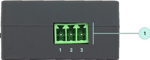
1. Terminal Connector for 2 wire RS485 connection and GND.
