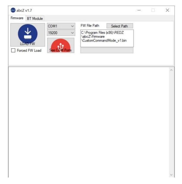
In order to use the software the specific firmware must be selected. After selecting the firmware path by clicking "Select Path" button the firmware can be loaded to device. The device has protection time window 10 seconds after the powered up so the process must be started within 10 seconds after the device powered up.
