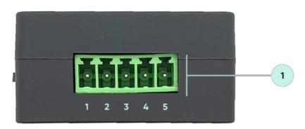
1. Terminal Connector for 2 wire RS485 connection and GND. Terminal also has external power input pins.
