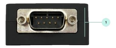
1. DB9 Male connector for RS232: Only Tx-Rx-GND for data transmission
