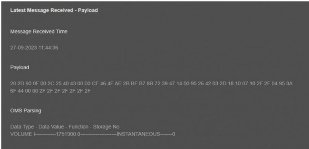
"Message Received Time": Shows the system time when this specific WMBus frame received.
