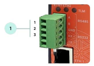
1. Terminal Connector for 2 wire RS485 connection and GND (if needed)
