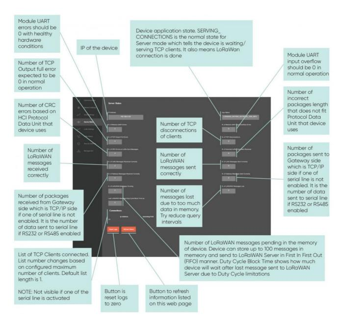
After clicking "Refresh Status" button, system will reload data only and will not reload page. Button will be disabled during reload for an instance. If timeout occurs during the reload, the button will be enabled again with warning of timeout. In normal operation reload of status data will be done immediately.
