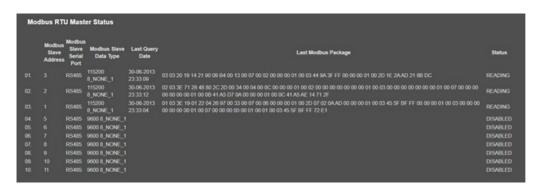
In this example all 3 queries are ok and we can see last messages from field device under Last Modbus Package column.
