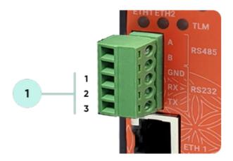
1. Terminal connector for 3 wire Tx-Rx-GND RS232 data transmission
