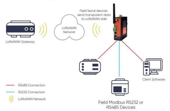
TLM Series LoRaWAN EndNode Modem set to Client Mode and device function set to Transparent. Field RS232 or RS485 devices such as PLCs and local software systems can make link with TLM over serial interface and can send data to LoRaWAN Server automatically.
