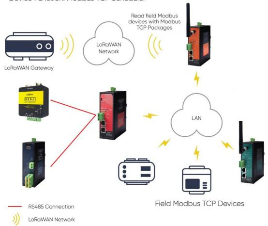
TLM Series LoRaWAN EndNode Modem set to Client Mode and device function set to Modbus TCP Scheduler. TLM can be connected to field Modbus TCP devices and it has built in mechanism to keep connection alive. Field Modbus TCP devices such as protocol converters, energy analyzers, PLCs and remote IO devices can be read by TLM Series LoRaWAN EndNode Modem and their data can be send to LoRaWAN Server automatically.
