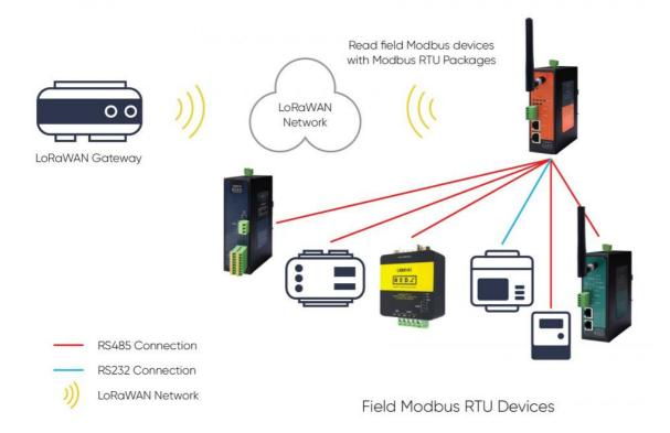
TLM Series LoRaWAN EndNode Modem set to Server Mode and device function set to Modbus RTU Scheduler. TLM can be individually connected to RS232 device and RS485 device, both serial interface can be active at same time. Field Modbus RTU devices such as protocol converters, energy analyzers, PLCs and remote IO devices can be read by TLM Series LoRaWAN EndNode Modem and their data can be send to LoRaWAN Server automatically.
