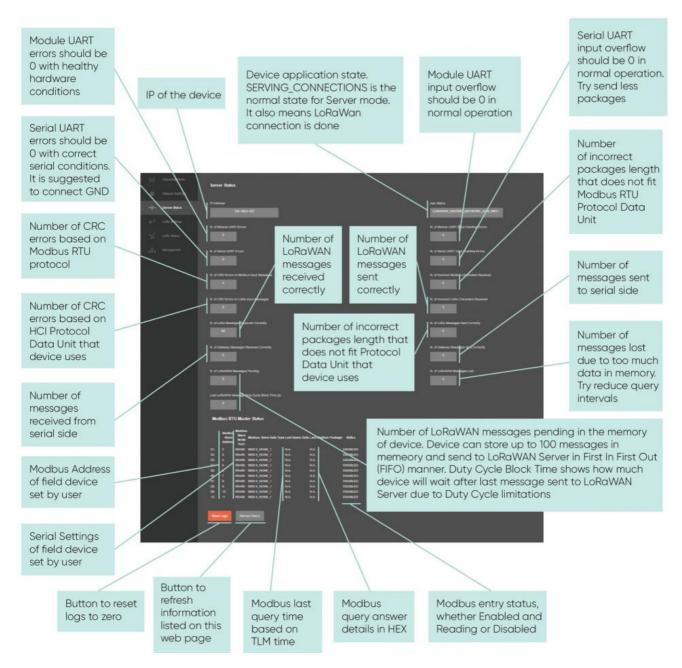
When device Function is set to LoRaWAN Transparent Modem, following page will be available:
