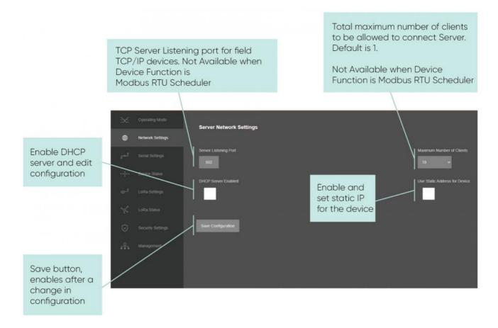
Following parameters and static IP settings available for "DHCP Server" setting.
