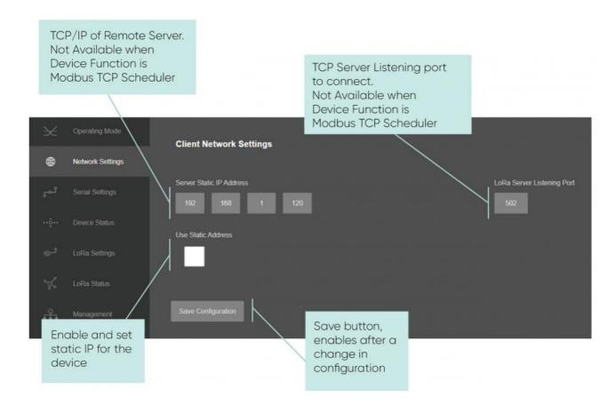
Following parameters and static IP settings available for "Use Static IP Address" setting
