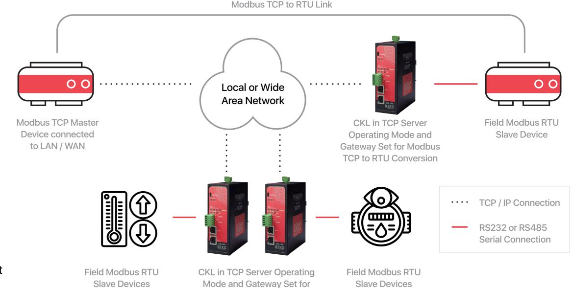
Modbus TCP to RTU Conversion
