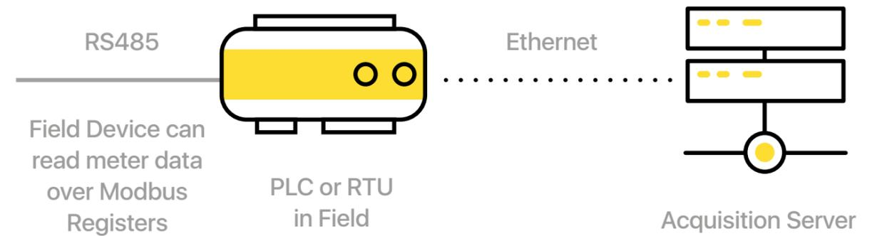
**LKM Series Modbus RTU to P1 Companion Standard Protocol Gateway is designed to be used with electricity meters that communicates in P1 Companion Standard**
