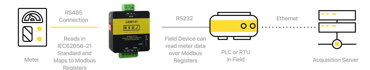
LKM Series Modbus RTU to IEC62056-21 Protocol Gateway are designed to be used with electricity meters that communicates in IEC62056-21 standard
