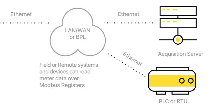
The meters that supports IEC62056-21 standard has read out tables that has several data such as import energy, export energy, phase voltages and currents. LKM Series Modbus to IEC62056 - 21 Protocol Gateway automatically reads that values and maps to Modbus registers. Field devices or software systems can easily read data over Modbus protocol so that energy meter reading can easily be integrated to field automation or monitoring systems without need of IEC62056-21 protocol implementation.
