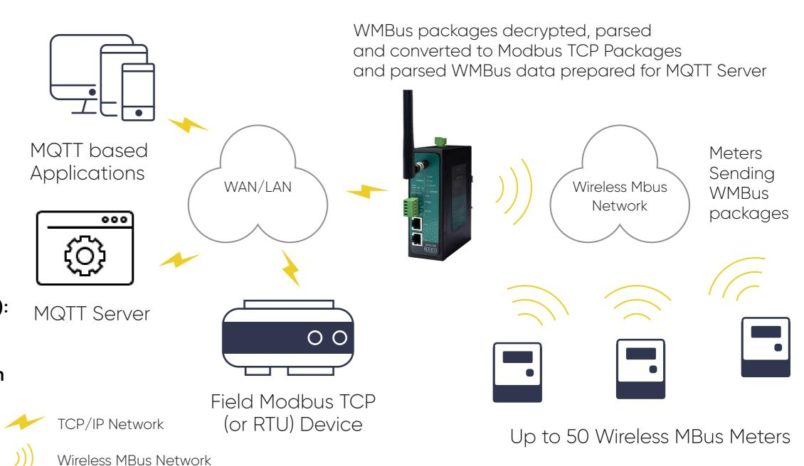
STG In all function modes 1-2-3-4-5-6: STG can decrypt up to 50 devices frames, for example in Function 6: Repeater function.
